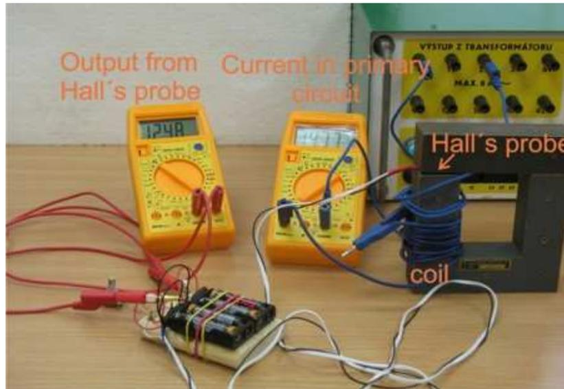
Fig. 3: Arrangement of the experiment
