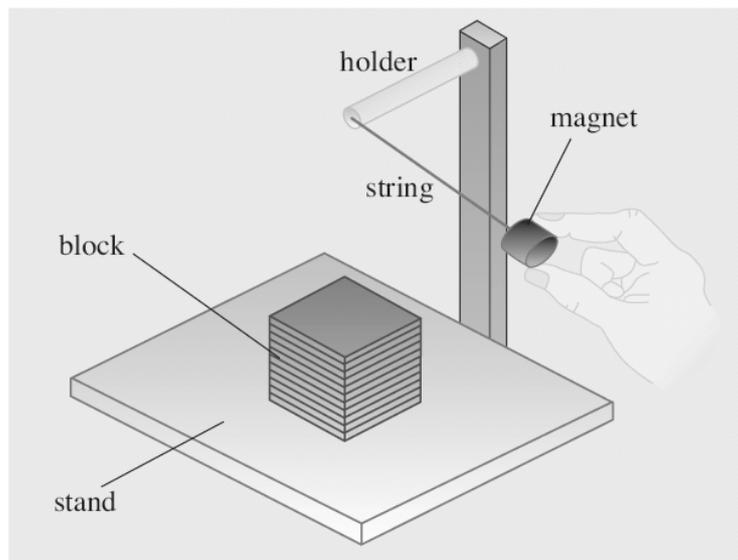
**Figure 4** Experimental setup of Magnetic pendulum experiment (figure is adapted from [11])
