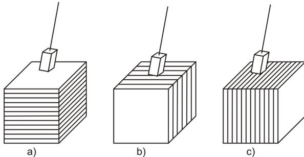
**Figure 5** Three orientations of the copper block in the experiment
