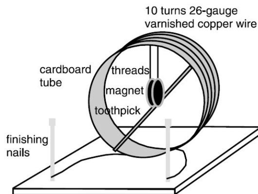
**Figure 2** Simple cheap ammeter (figure is adapted from [3])
