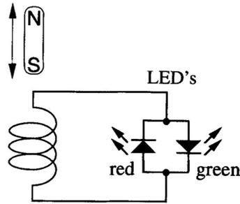
**Figure 3** LED's used to study electromagnetic induction (figure is adapted from [4])
