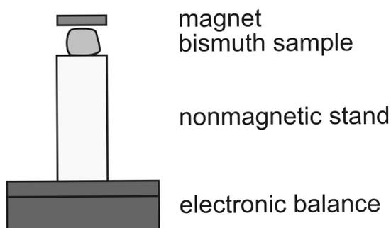
**Figure 1.** The arrangement of the experiment “Demonstrating diamagnetism”
