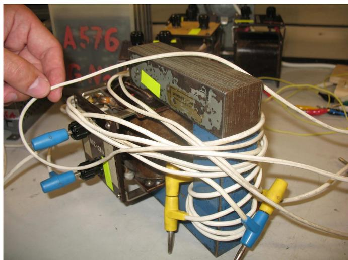
**Figure 5.** The result of an experiment how to make assigned voltage in the secondary coil of electric transformer (voltage, which would require non-integer number of turns in the secondary coil)
