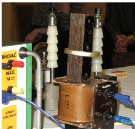
**Figure 7.** Levitating ring
