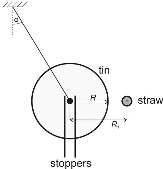
**Figure 2.** Arrangement of the experiment (viewed from the side)
